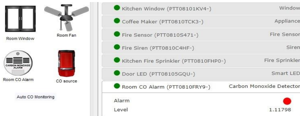
Figure 4.40. The room window is closed and the room fan is OFF after the CO level is less than 2%.
