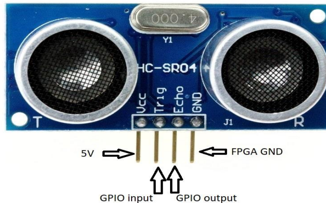
Figure 3.7: Ultrasonic sensor connections.
