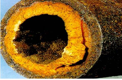
Figure 1 : DEPOSITION DE PARAFFINE DANS LES CONDUITES
