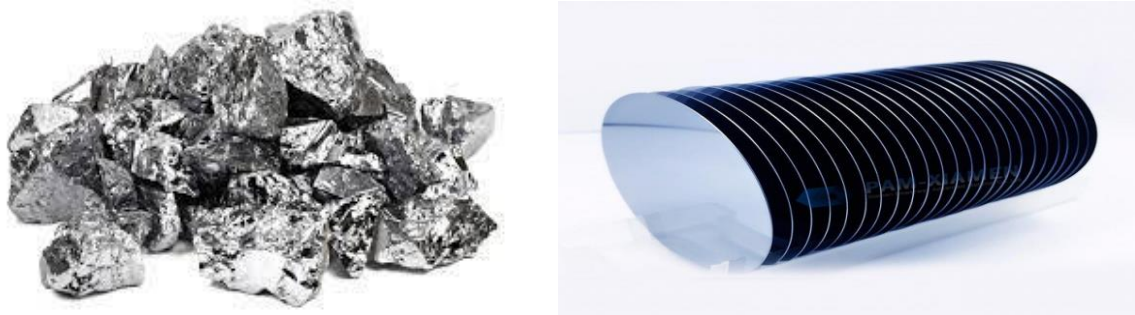
Figure 2.9 From a Silicon rock to wafers
