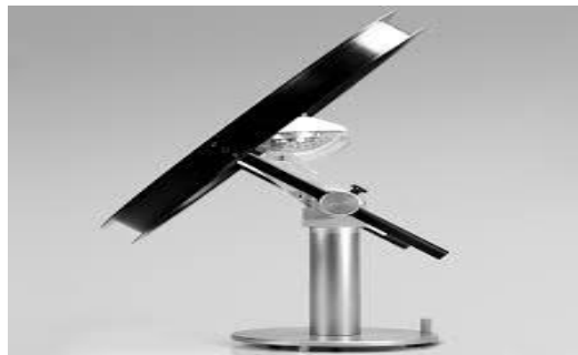
Figure 2.7 Pyranometer with a shadow ring
