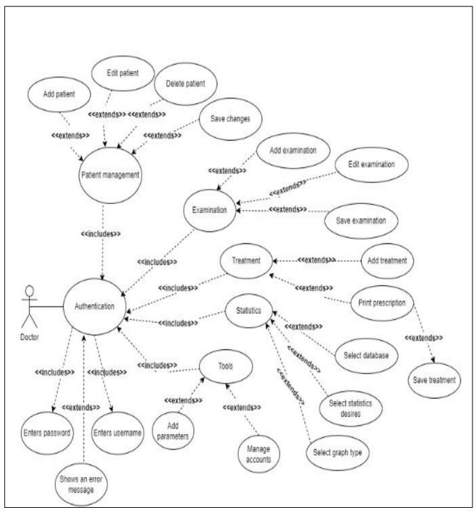
Fig 2. 3 Doctor's use case diagram
