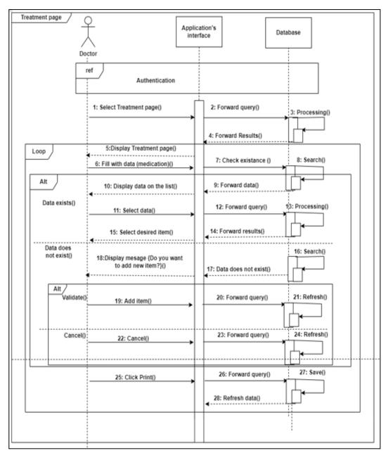
Fig 2. 11 Treatment's sequence diagram
