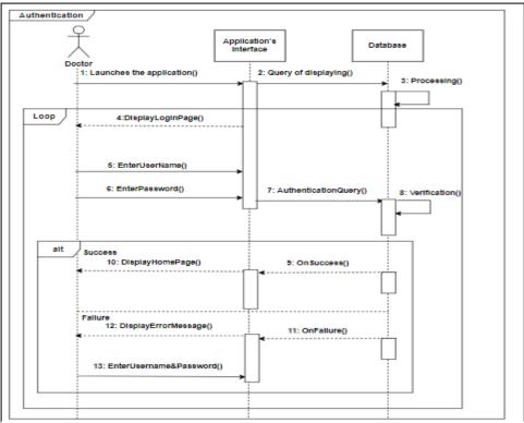
Fig 2. 7 Authentication's sequence diagram
