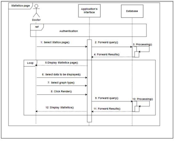
Fig 2. 12 Statistics' sequence diagram
