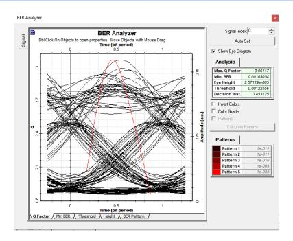
Figure 3.5: eye diagram of channel 1 in 4-channel WDM
