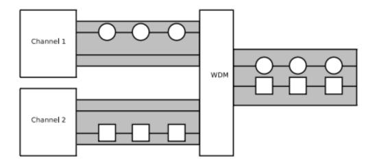
Figure 1.9: Simple schematic of a WDM system for N = 2
