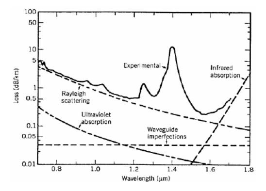
Figure 1.8: Optical fiber attenuation curve
