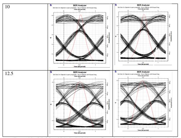
From tables 3.7, 3,8 and 3.9, the 75-25 km configuration gives higher Q factor and wider eye diagrams in all channels for the 5Gbps and 10Gbps bit rates, and in ch-1 and ch-8 for 2.5Gbps. Hence for the others bit rates the 100 km configuration results are better except in ch-16 for 12.5 Gbps.
