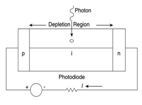
Figure 1.6: PIN photodiode
