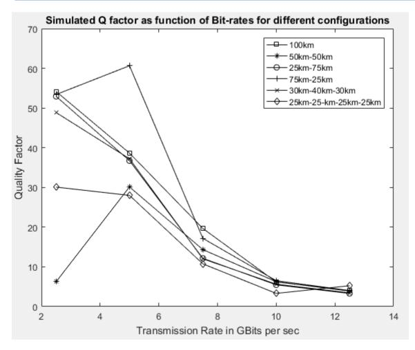
Figure 3.13 : Simulated Q factor as function f Bit-rates for different configurations
