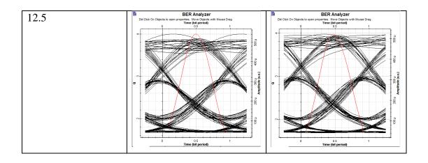
From tables 3.4, 3,5 and 3.6, in channel 1 and channel 8 the 75-25 km configuration gives better results for 2.5Gbps and 5Gbps we have got higher Q factor and wider eye diagrams but as a higher data rate is transferred, the 100 km configuration Seems more convenient for the same channels. In the other side, the results obtained in channel 5, for 2.5 Gbps and 5 Gbps the 100 km configuration are slightly better and vice versa for the other bit rates.
