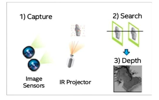
Figure 2.9. Active Infrared (IR) Stereo Vision Technology [16].
