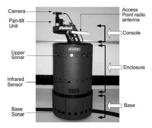
Figure 2.1: The B21r mobile robot.
