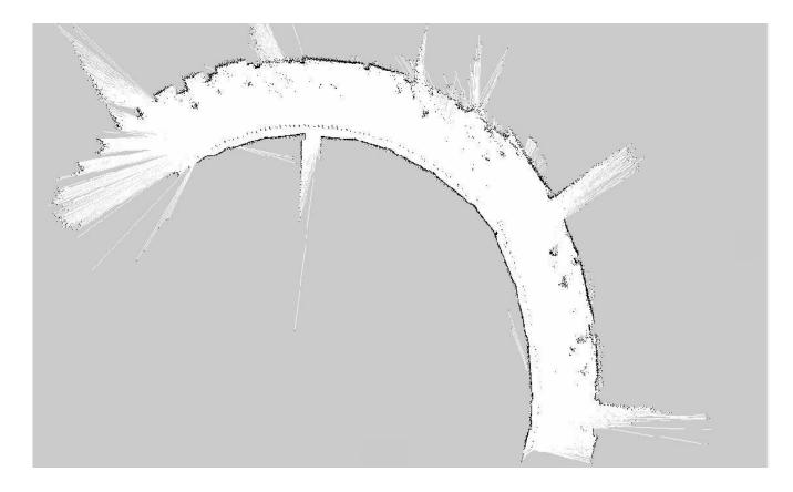
Figure 4.3. map of the CDTA hallway using Gmapping SLAM
