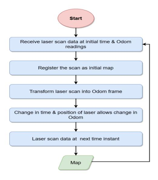
Figure 3.5. Gmapping Slam flowchart.
