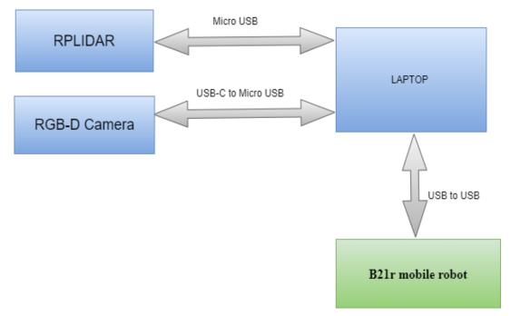
Figure 2.11. Schematic diagram of our mobile robot.
