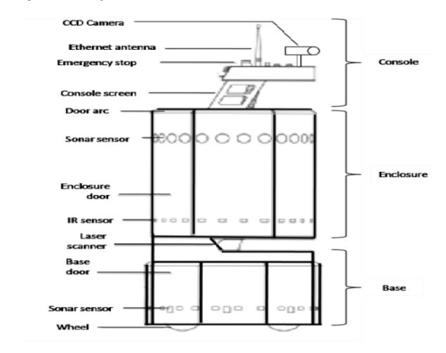
Figure 2.2: The B21r and its onboard sensors.
