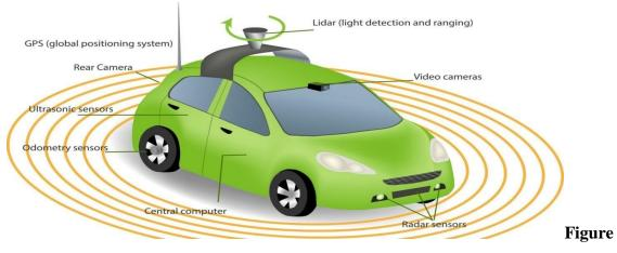
1.8. Mobile robot equipped with various sensor types [7].
