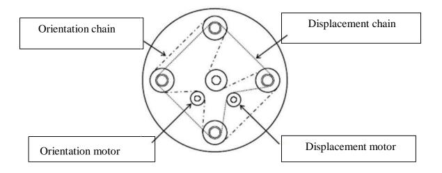
Figure 2.3: The platform geometry of a synchronous drive mobile robot.
