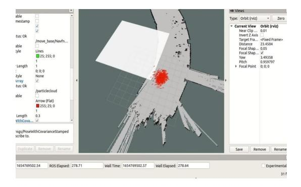
Figure 3.12. Particle localization
