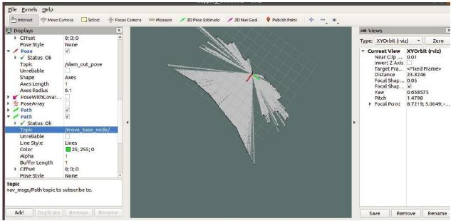
Figure 3.8. Hector-SLAM on rviz using lidar
