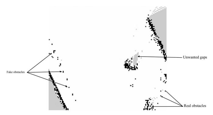
Figure 4.5. different errors may happen when mapping
