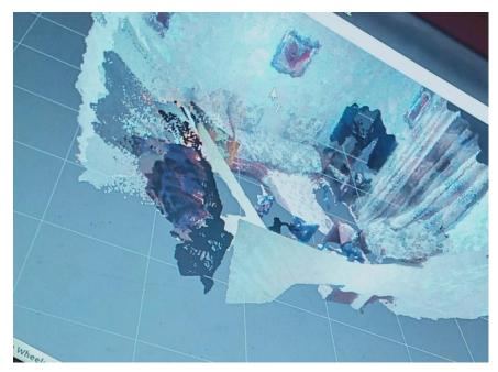
Figure 3.10. Starting visual slam with d435i camera.
