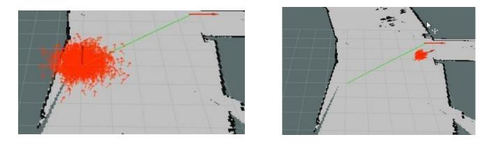
Figure 4.7. AMCL localization results. (a) Cloud in starting pose. (b) Cloud in final pose.
