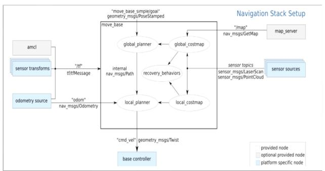
Figure 1.15. Overview of a typical system running the Navigation Stack [15].
