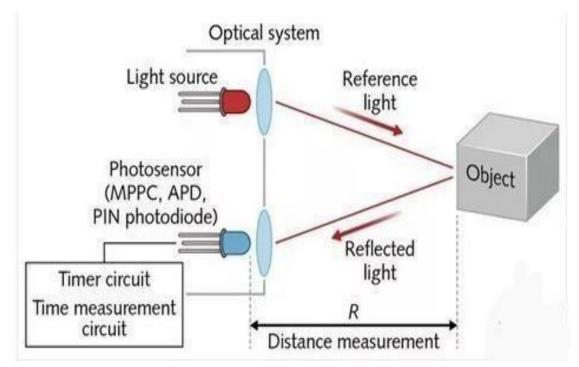
Figure 2.7. TOF ranging schematic [15].
