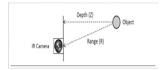
Figure 2.10. Depth Measurement (Z) versus Range (R) [16].
