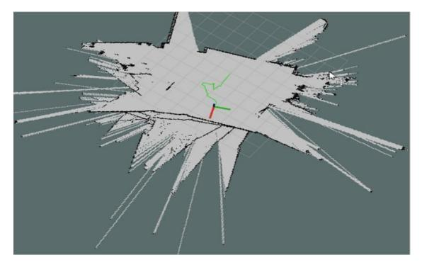
Figure 4.6. Error caused by sudden moves.
