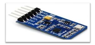
Figure 1.12. Inertial measurement unit (IMU)
