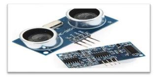
Figure 1.10. HC-SR04 Ultrasonic sensor
