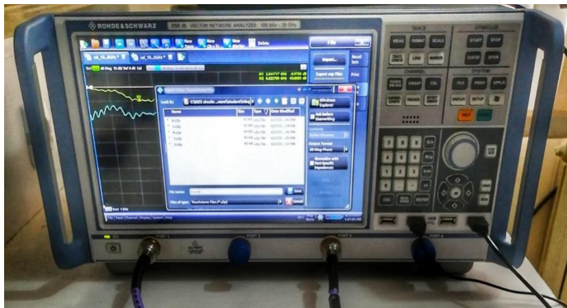
Figure 3.23 Vector Network Analyzer used for measurement
