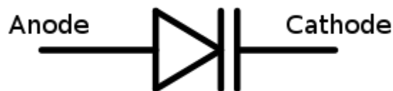
Figure 1.11 Varactor electronic symbol
