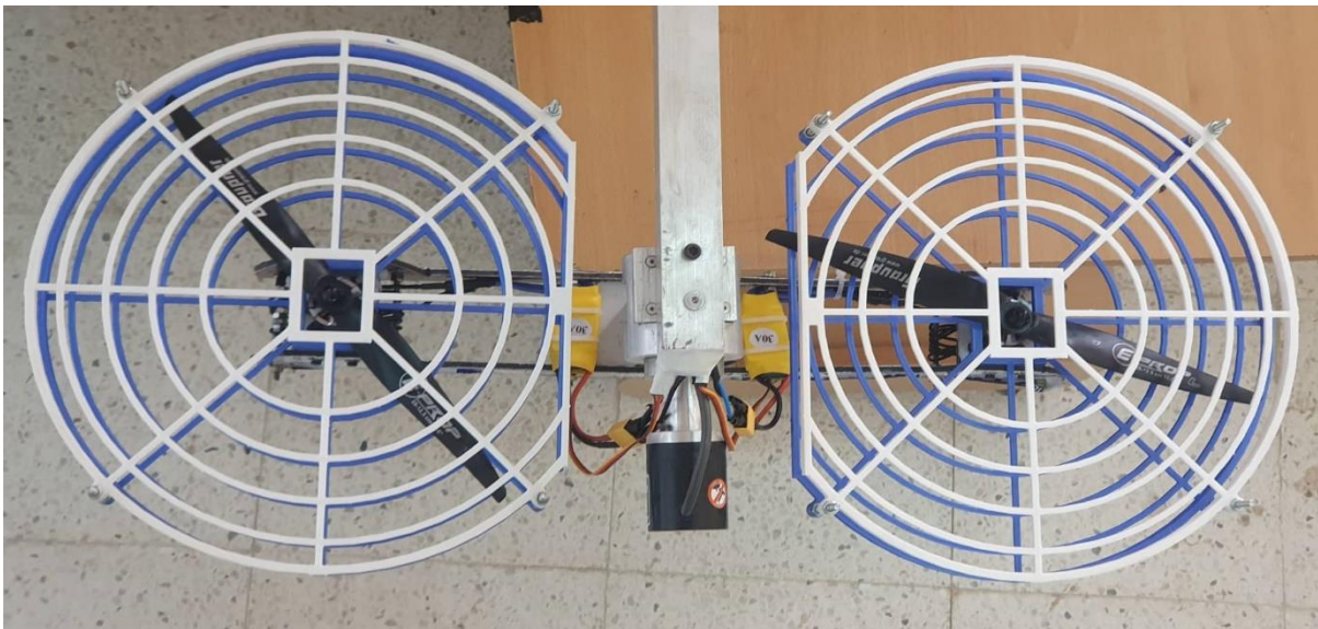
Figure5.19: Protection implementation In lab
