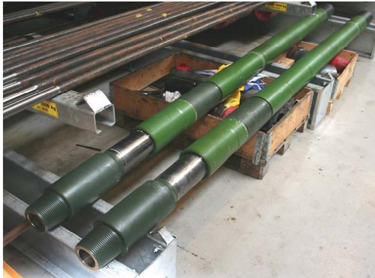
Figure II. 14: Anti Stick-slip Tools ASST
