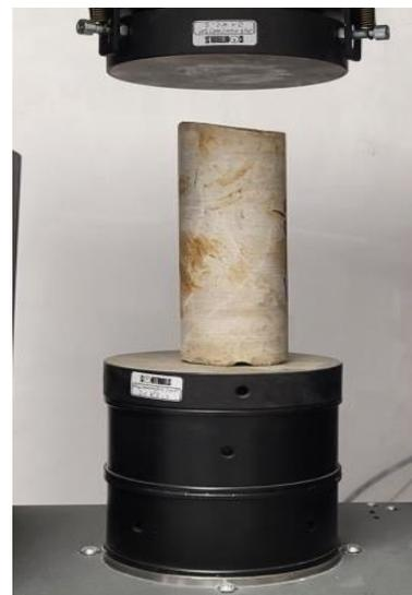
Figure IV-6 : Test de compression non confinée (Zhug, 2019)
