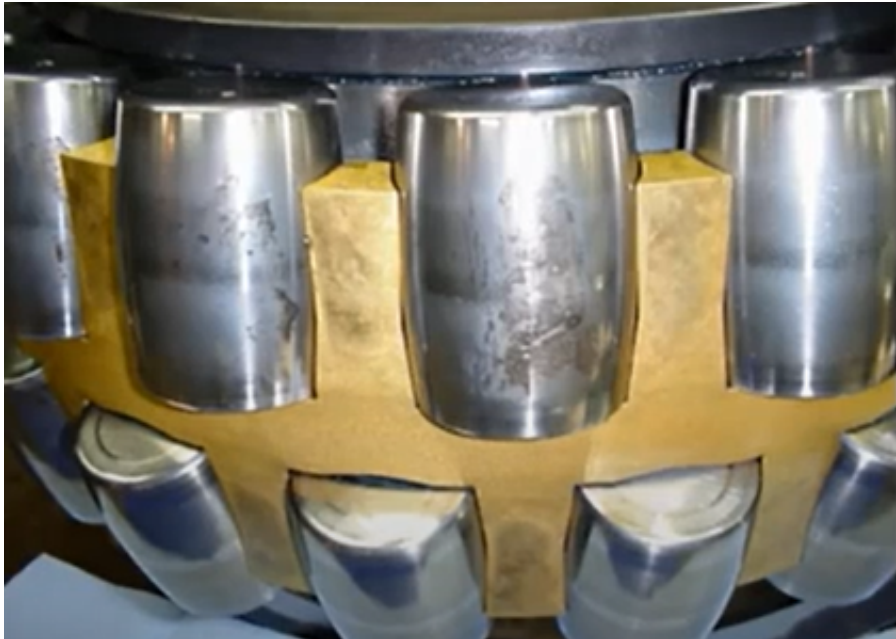
FIGURE 3.22 – dommage subsurfacique des roulements
