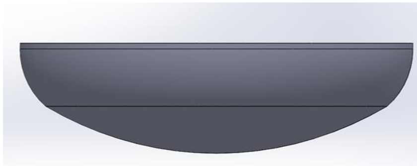
FIGURE III-7: FOND INFERIEUR APRES REVOLUTION
