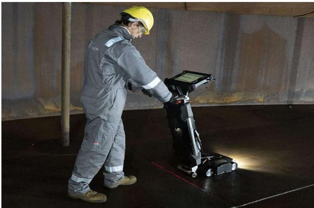
**Figure III. 14: MFL surface scanner**
