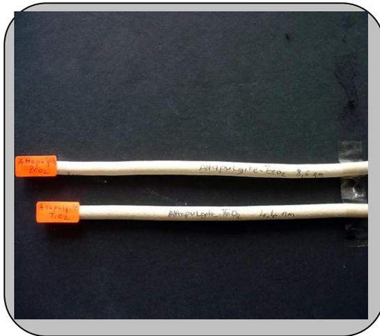
**Figure 46:** Supports Attapulgite/ZrO<sub>2</sub> et Attapulgite/TiO<sub>2</sub>
