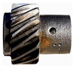
Figure 22: Gear corrosive wear
