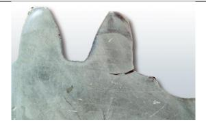
Figure 25: Tooth crack
