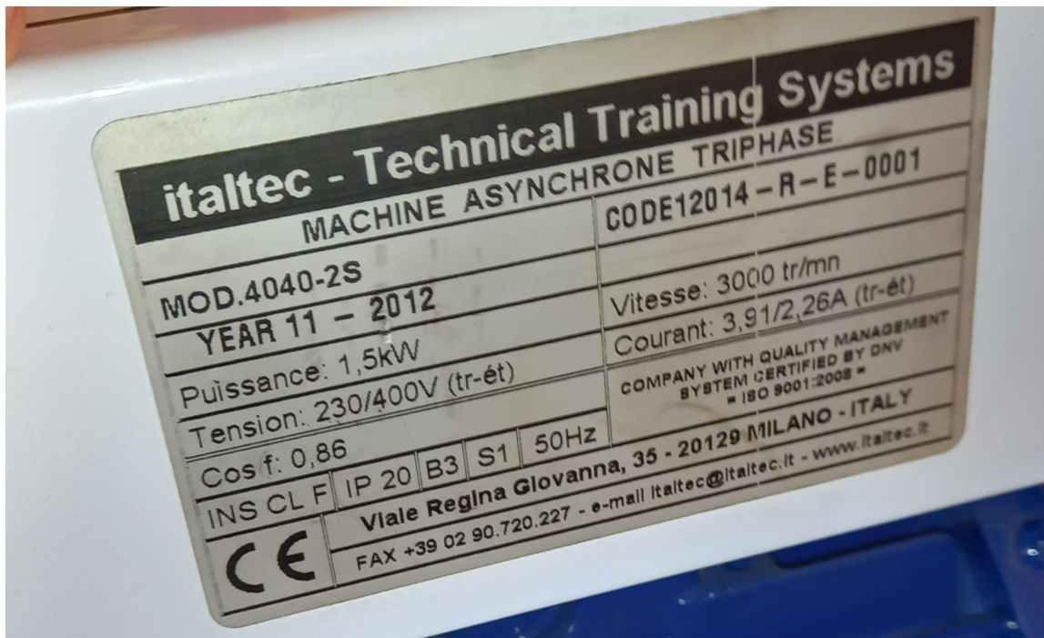
Figure 3.1: Nameplate of the used induction motor
