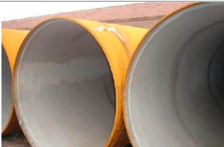
Figure III. 2 Cement coating for the internal surface of the pipes.
