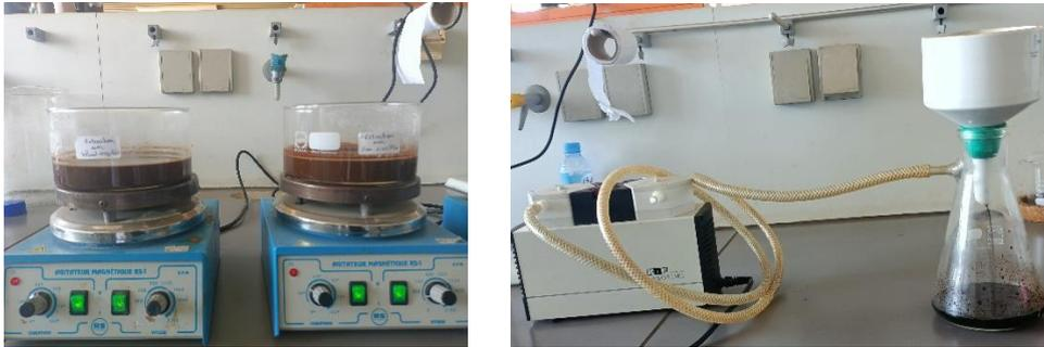
**Figure III.21.** Purification de la lignine
