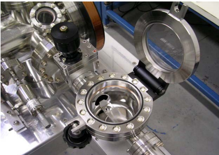
Figure 2.2.14: Close up of the load lock, showing the demountable sample holder
