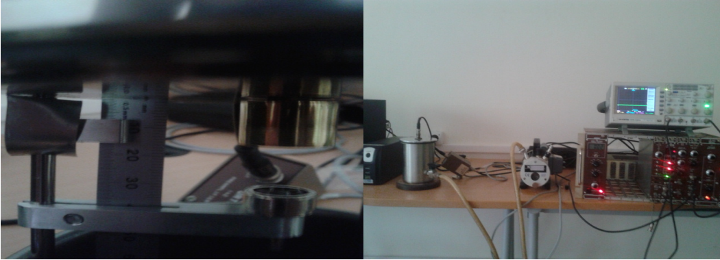
Figure 4.4.5: Vacuum chamber+ Irradiation set-up of the third series CR39(\neq E^*)
