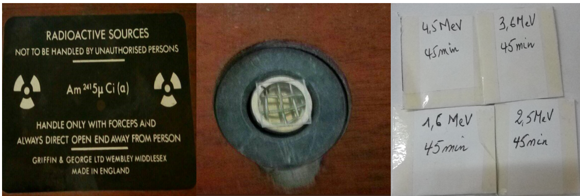
Figure 4.4.3: ^{22}Na radioactive source + ^{241}Am source+CR39 samples
