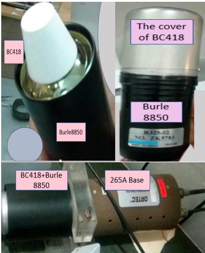
Figure 2.1.9: The composed detector of BC418+Burle8850+265A Base
