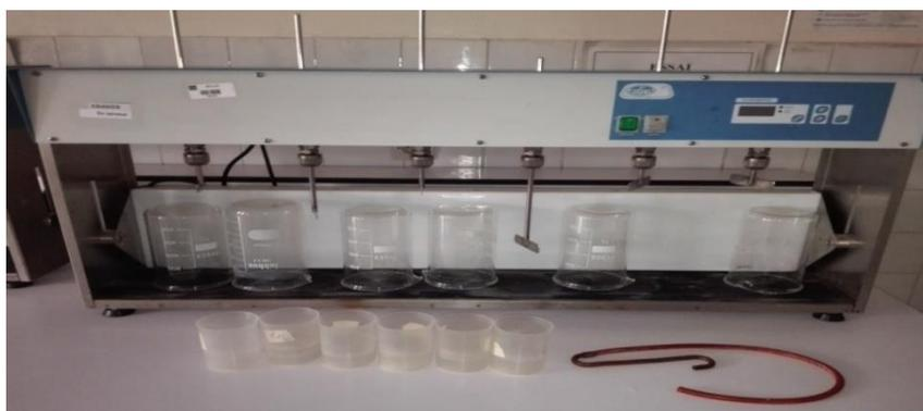
**Figure V-12 :** Jar test.
