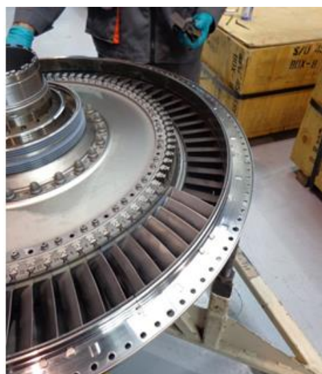
Fig.12 a) Distribution of the blades on the disk by numbering of the blades in order of the results, b) View of a rotor disk during assembly of the blades in order of the results of the static distribution
