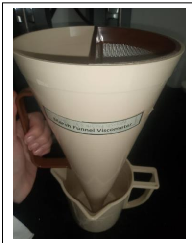
Figure II-12 : Marche Funnel Viscometer
