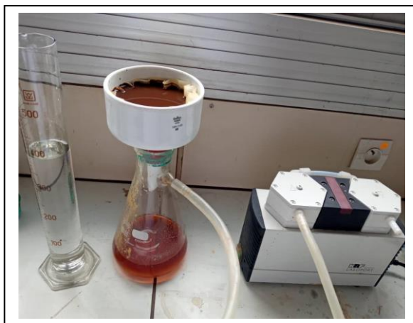
Figure II-21 : Purification de la lignine
