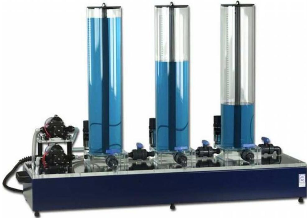
**Figure 5.44** Station DTS-200 (three tank system)
