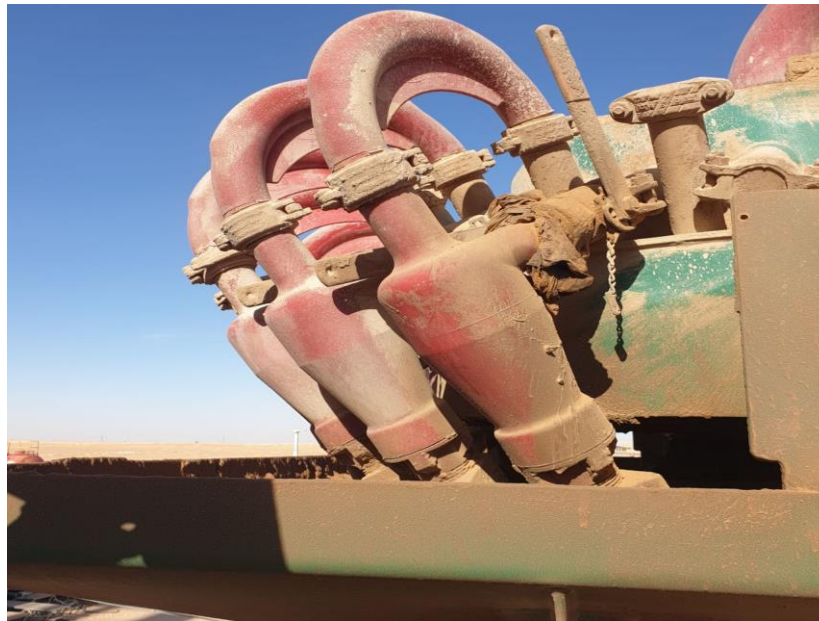
Figure 1.9: Desilter de mud cleaner RIG ENF#61 la marque derrick.
