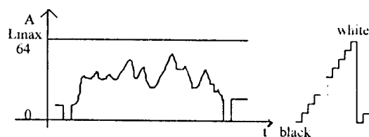
Fig-4.3 One-dimensionnal A-mode line signal
