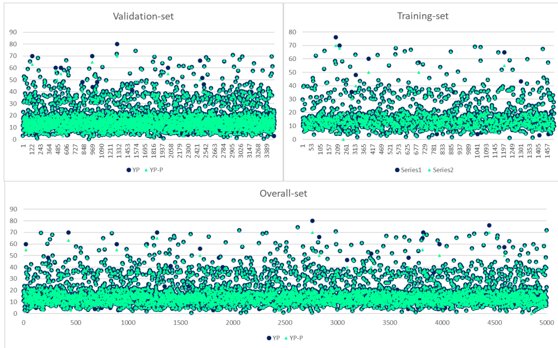
Figure 5-27 M-YP Model Predictions vs. Actual Yield point: Training, Testing, and Overall Results
