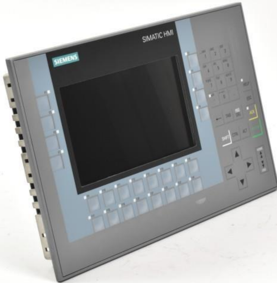
Figure 4.2. KP1200 COMFORT Tactile panel
