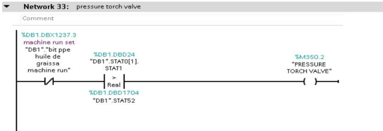
Figure 3.21. The network of pressure torch valve condition
