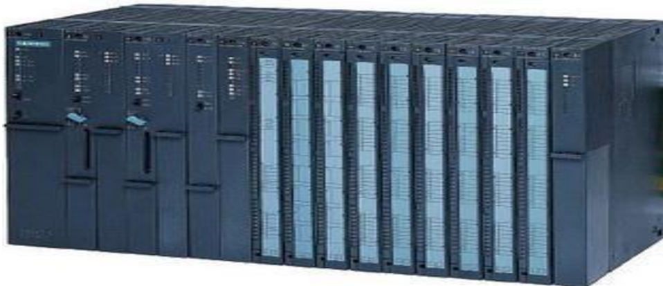
Figure 3.3. Siemense PLC S7-400
