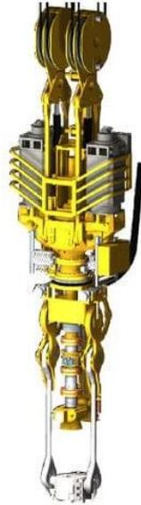
Figure I. 14: système top-drive.
