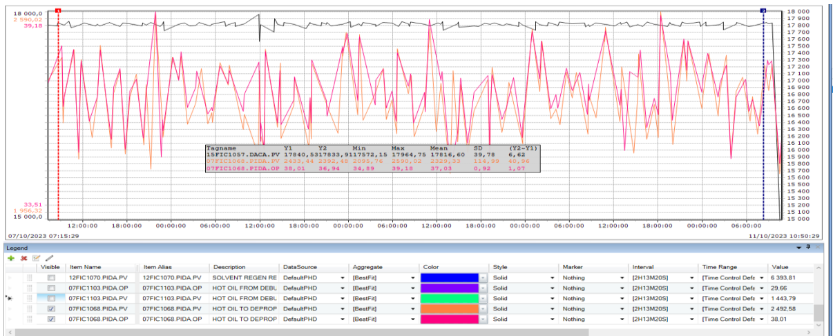
Figure IV.32 : Oil Flow Rate Trend of the 07MC04 Reboiler in the Depropanizer Column After APC Installation
