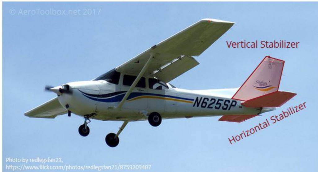
Figure II.5 A Cessna 172 with the Horizontal and Vertical Stabilizer Labelled [19]
