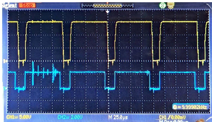
Fig.III.14b. Duty cycle signal of 83%.
