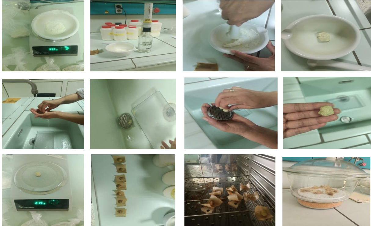
Figure 17: Equipment used for determining the wet and dry gluten content (by manual method)
