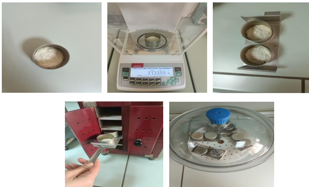
Figure 12: Equipment used for determining water content
