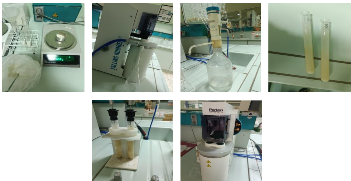
Figure 16: Equipment used for determining the Hagberg-Perten Falling Number Index
