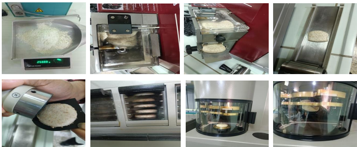
Figure 18: Equipment used for determining the Alveograph test
