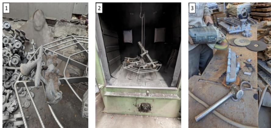
*Figure IV-20 : (1), (2) Grenailage et (3) finition.*
