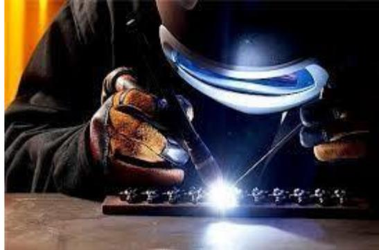
*Figure II.16: Soudure TIG.* [11]
