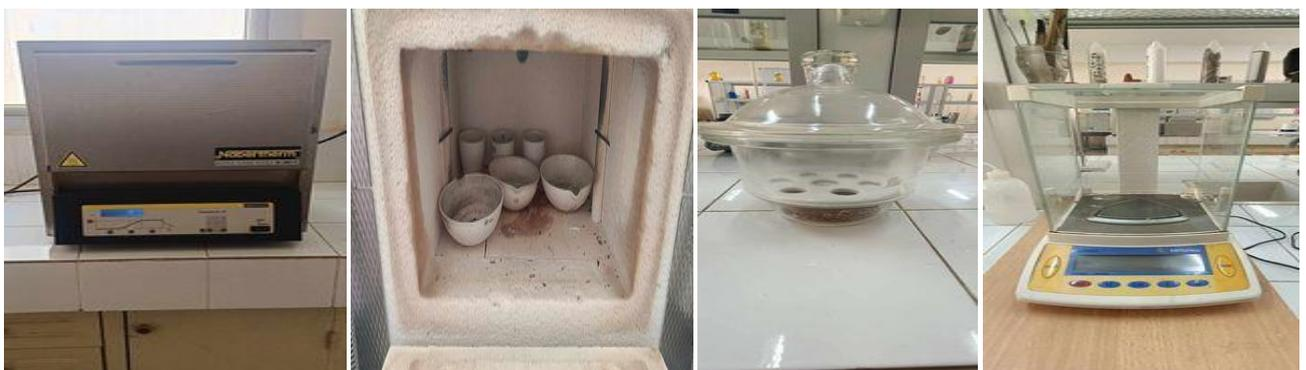
Figure 6 : Four a moufle, capsules, dessiccateur, balance
