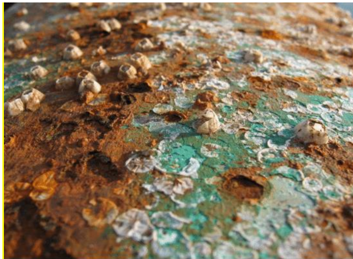
Figure II.3 La corrosion biochimique
