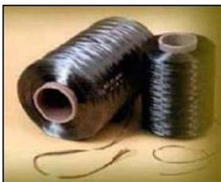
Fig.I.3. Bobine de fibre carbone
