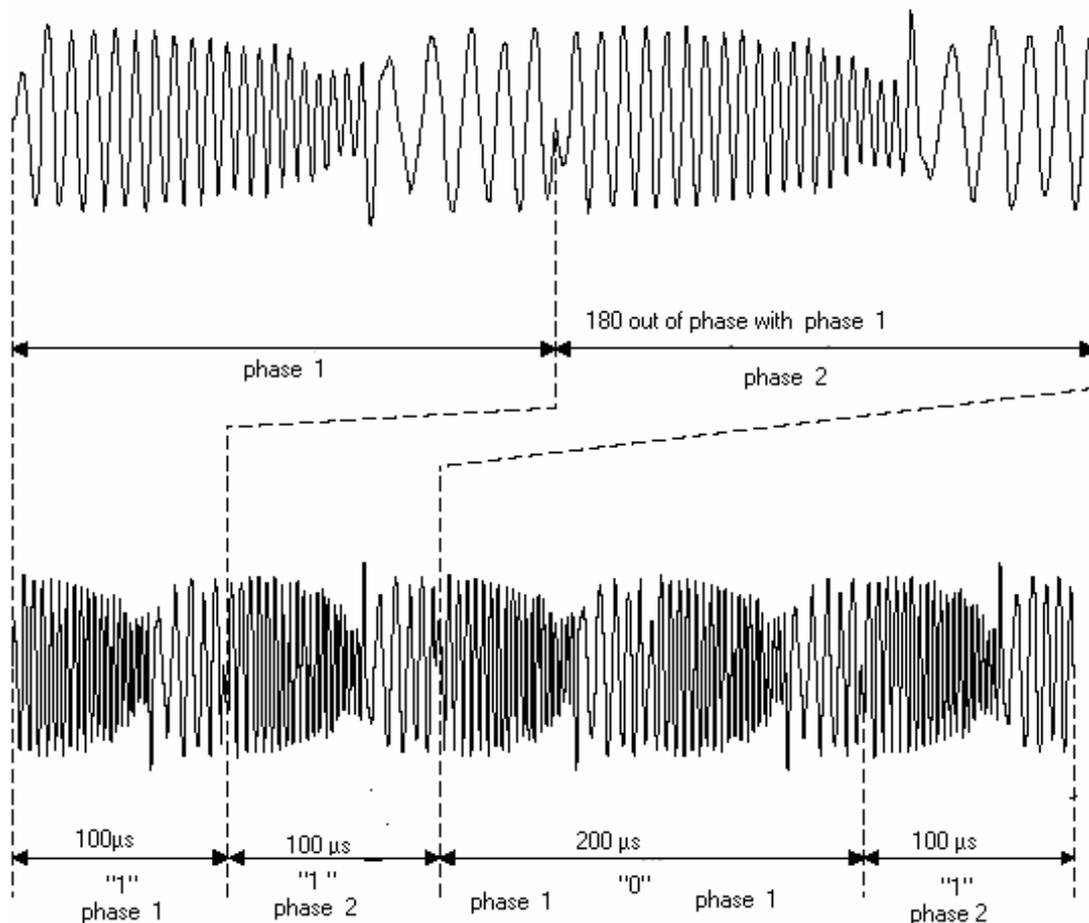
**Figure 3.4 Phase Reversal Keying (PRK) Data Pattern**
