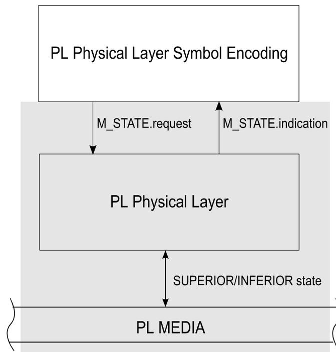
**Figure 3.7 Powerline Lower Layers Relationship [22]**
