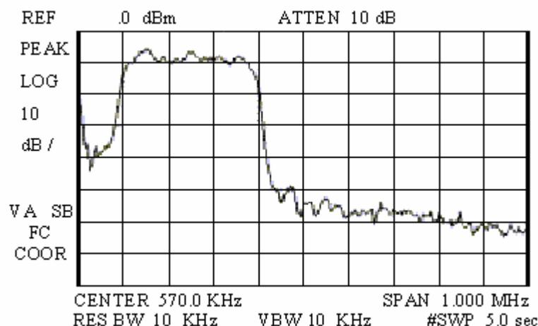
**Figure 3.2. Frequency Spectrum of a PL “Chirp” [1]**
