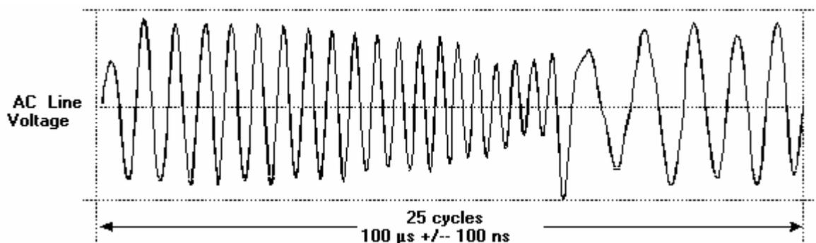
**Figure 3.5 Frequency Swept Carrier Waveform**
