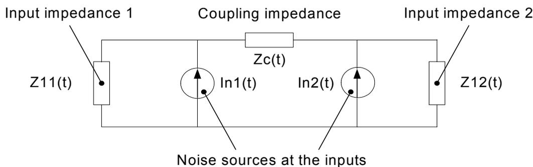
**Figure 2.2 Dostert’s Power Line Channel Model [18]**
