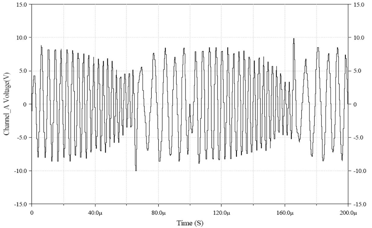
**Figure 5.4 transmission of two consecutive “1” in a packet message.**
