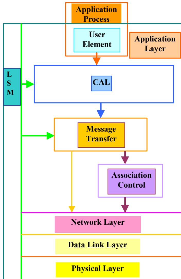
Figure 4.5 Application Layers Interfaces.
