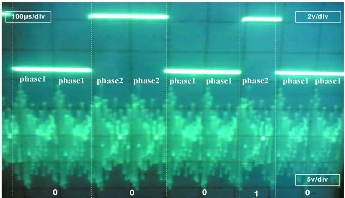
**Figure 5.7 Packet Transmission of 00010**
