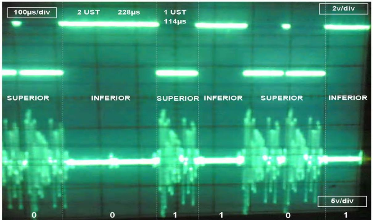
**Figure 5.6 Preamble Transmission of 001101**
