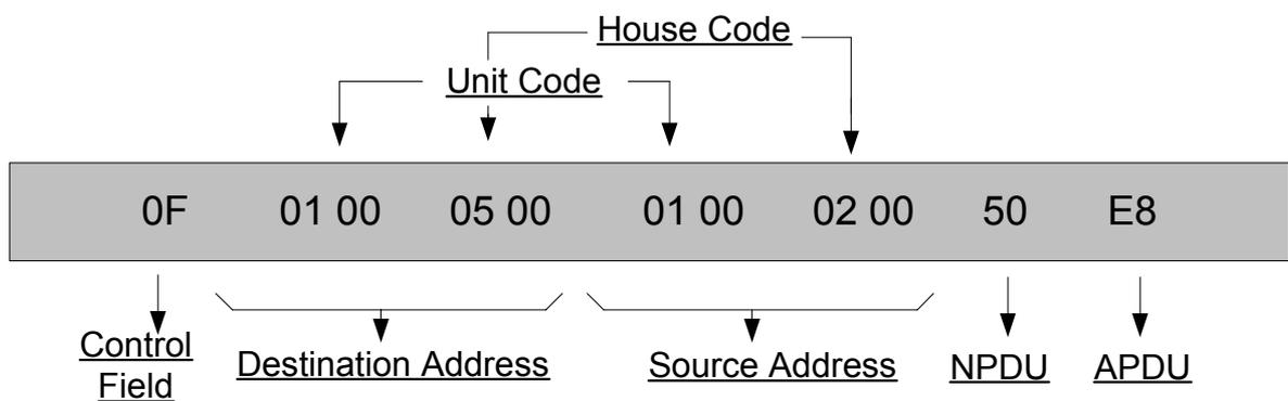
The first byte is the Control Field of the LPDU header as shown on Figure 5.6. The next four bytes are the destination address followed by the source address in right to left order. These addresses along with the Control Field make up the LPDU header. The next two bytes are the NPDU and the APDU headers.
