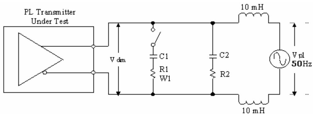
**Figure 3.6 Carrier Output Voltage Test Circuit [21].**
