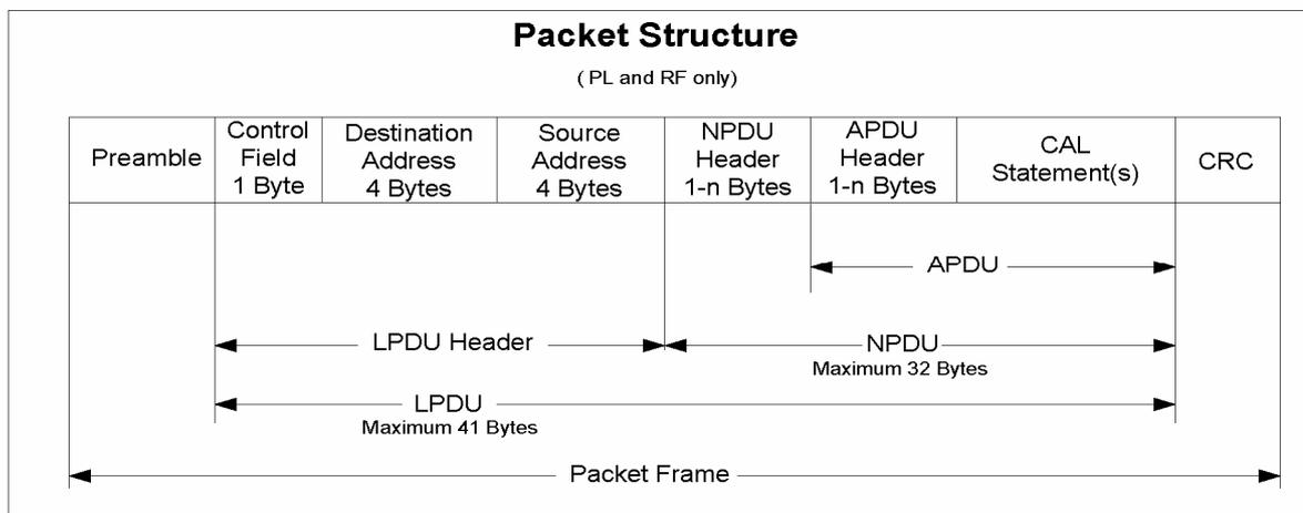
**Figure 5.13 Packet Structure**
