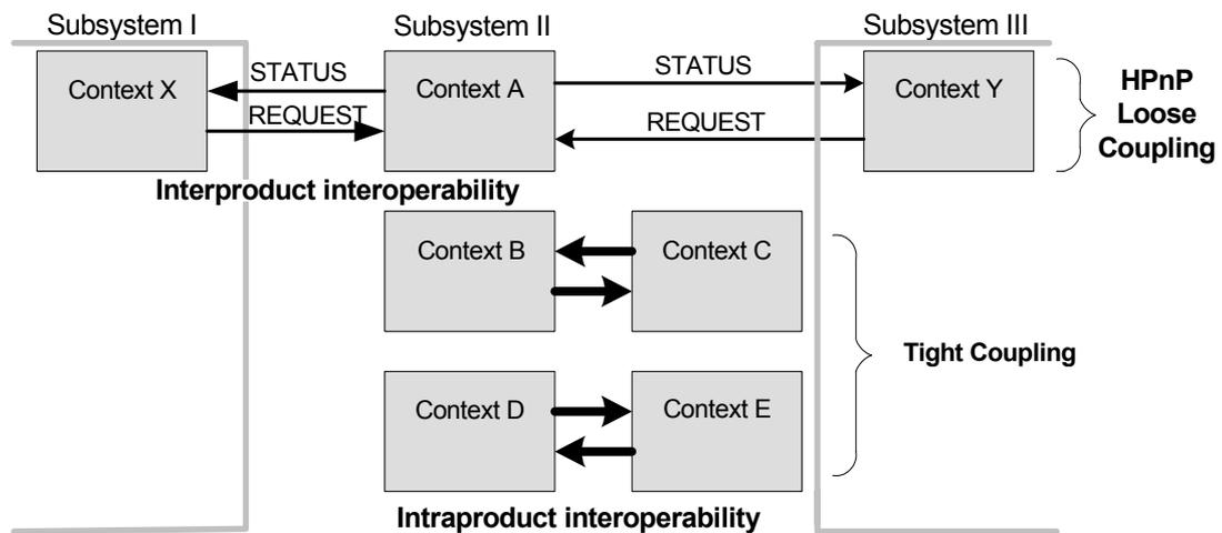
**Figure 4.11 Basic model of inter and intra subsystem interoperability**
