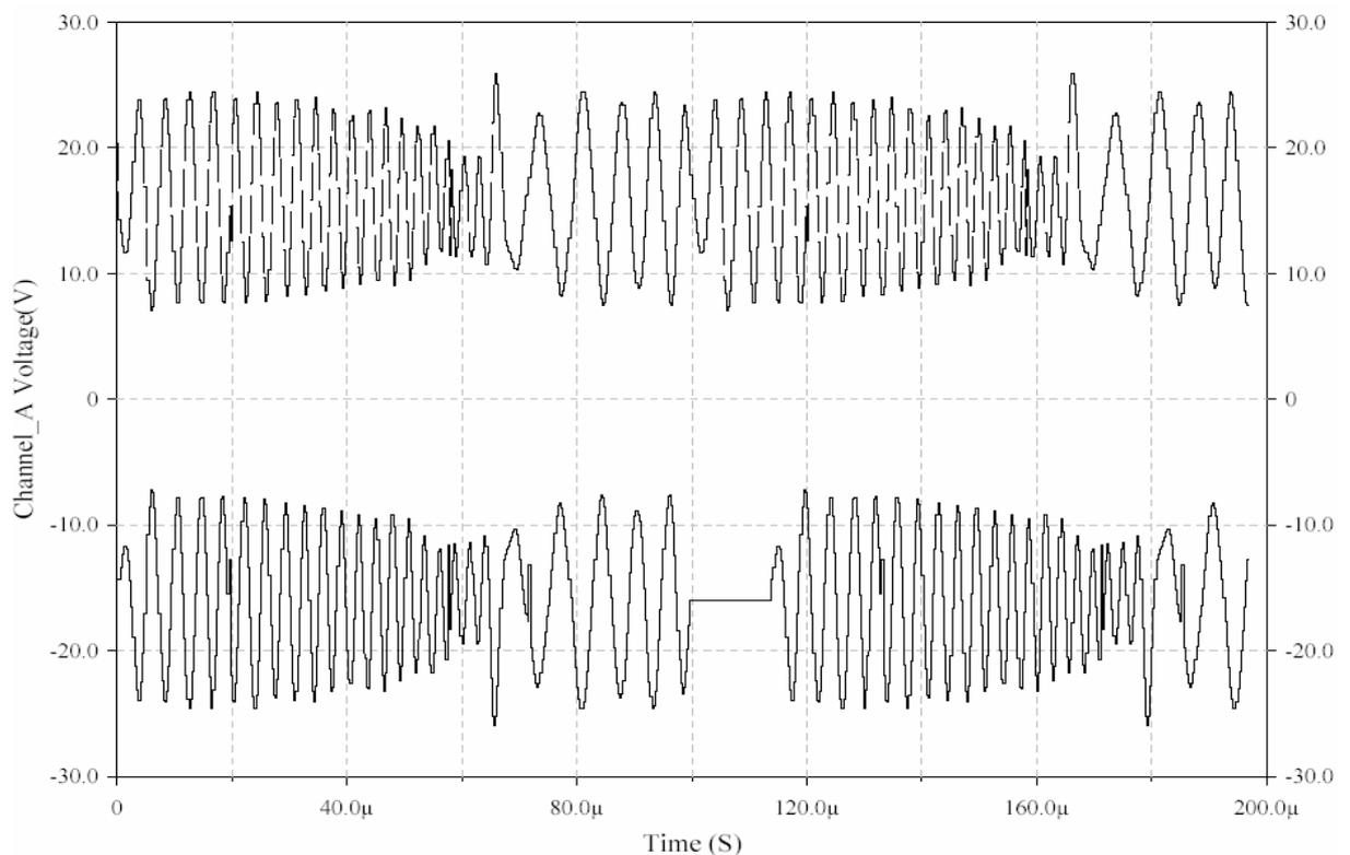
**Figure 5.3 PRK and ASK modulation of symbol “0”.**
