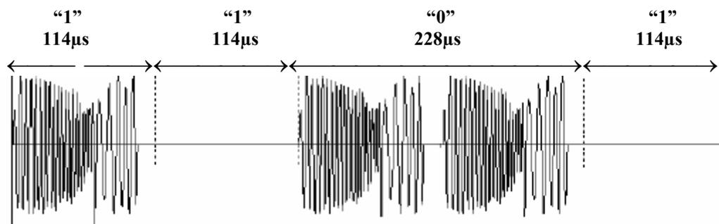
**Figure 3.3 Amplitude Shift Keying (ASK) Data Pattern**
