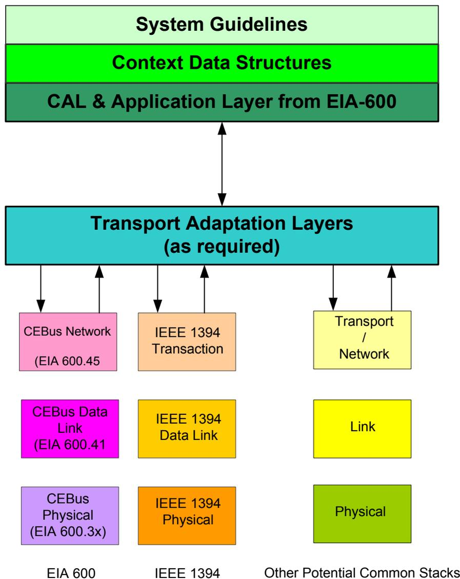
Figure 4.4 Application Diagram Supporting HomePnP on Multiple Stacks.
