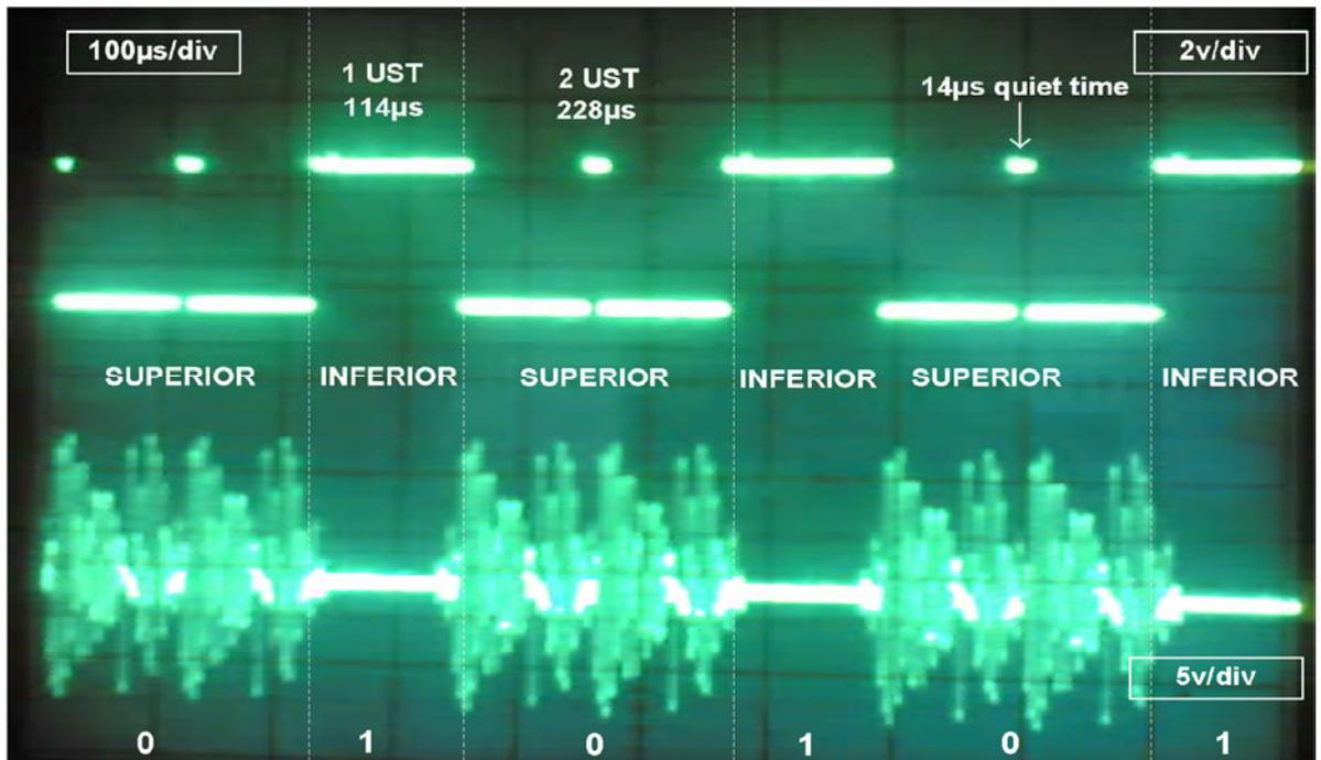
**Figure 5.5 Preamble Transmission of 010101**
