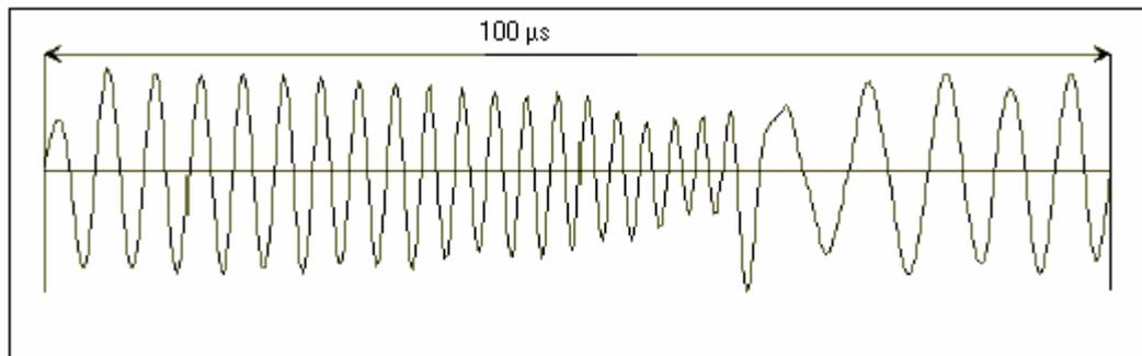
**Figure 3.1 Spread Spectrum Carrier Chirp**
