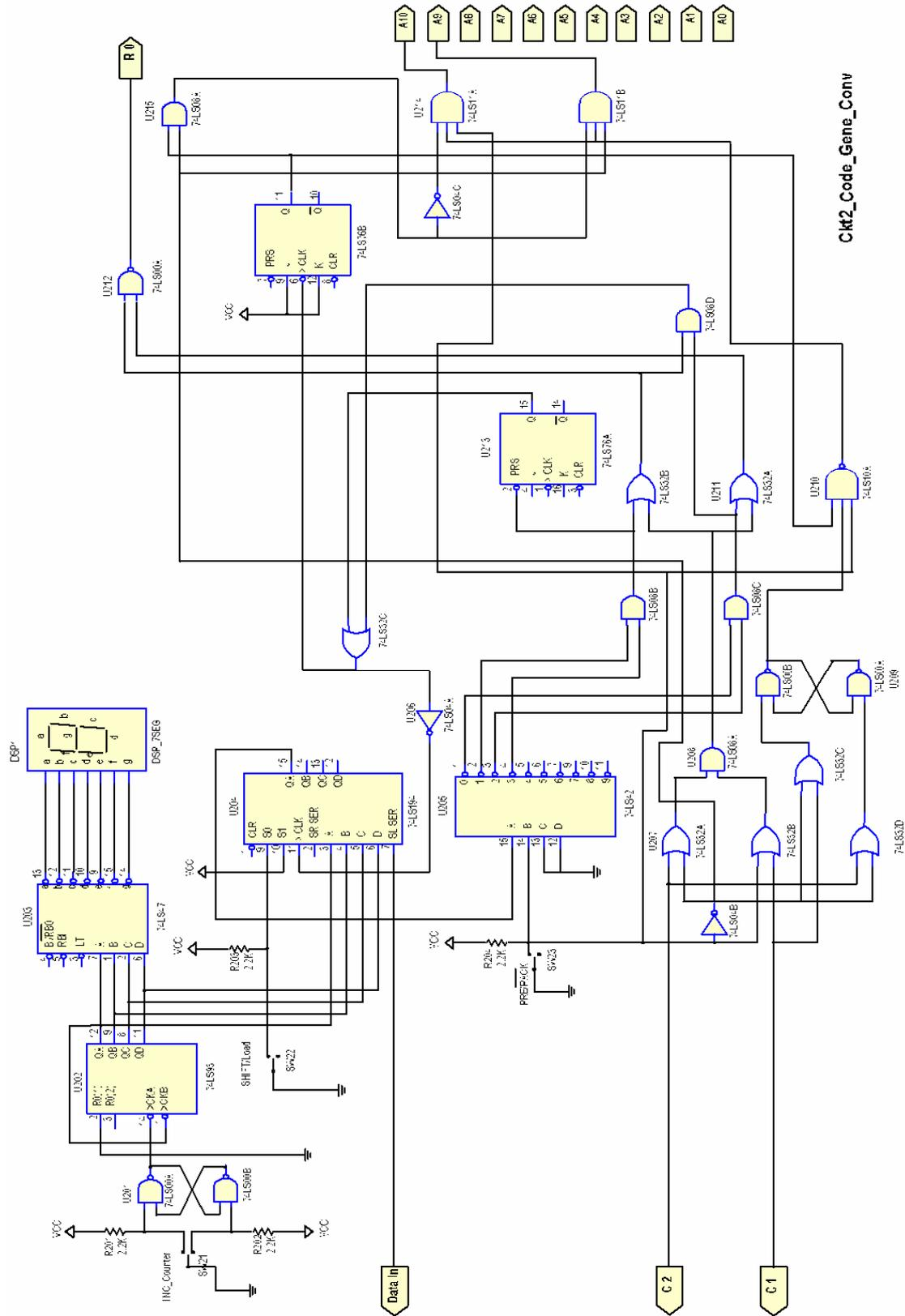
Fig 6.10 Code generation and conversion circuit
