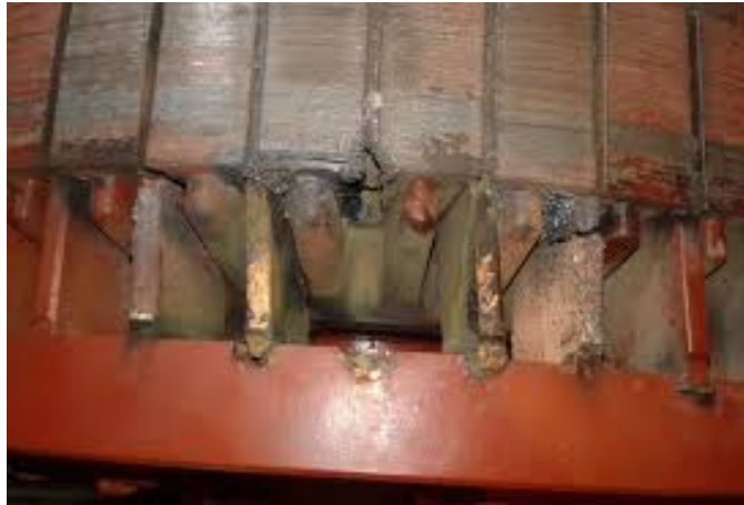
Figure 1.6: Broken rotor bar [18].
