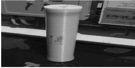
Figure 1.12 Typical 8-in. membrane element [1].
