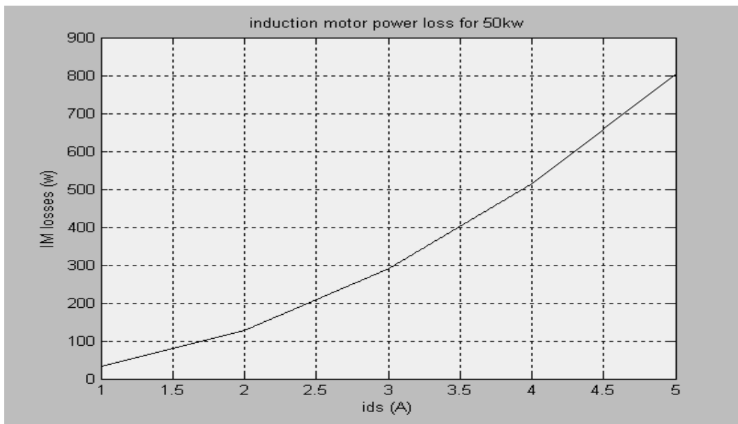
Fig.5.2. Variation of Total Losses with Current-Flux Component for 7.5 kW and 50 kW Induction Motor.
