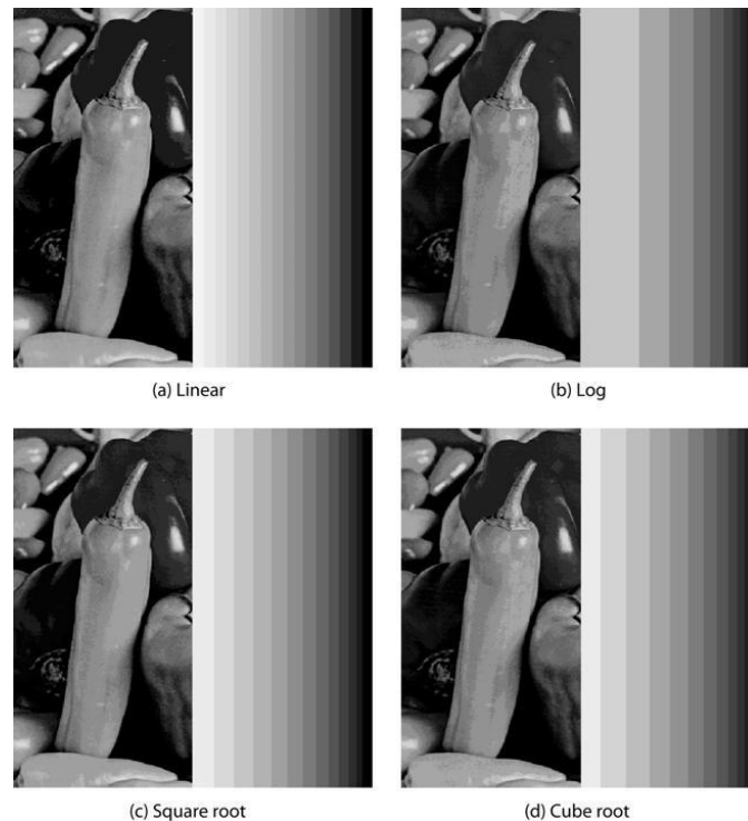
Figure 1. 6 Comparison of lightness scale quantization of the peppers_ramp_luminance image for 4 bit quantization
