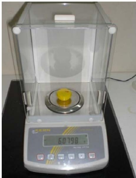
Fig. V.4: Balance analytique (Kern ALS 220-4)
