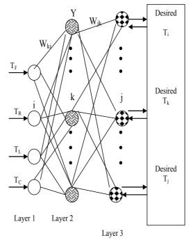
Fig. 4 Target Localization Neural Network
