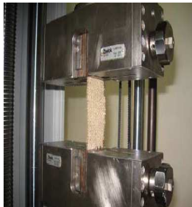
Figure 3. Tensile test of reinforcing jute fabric
