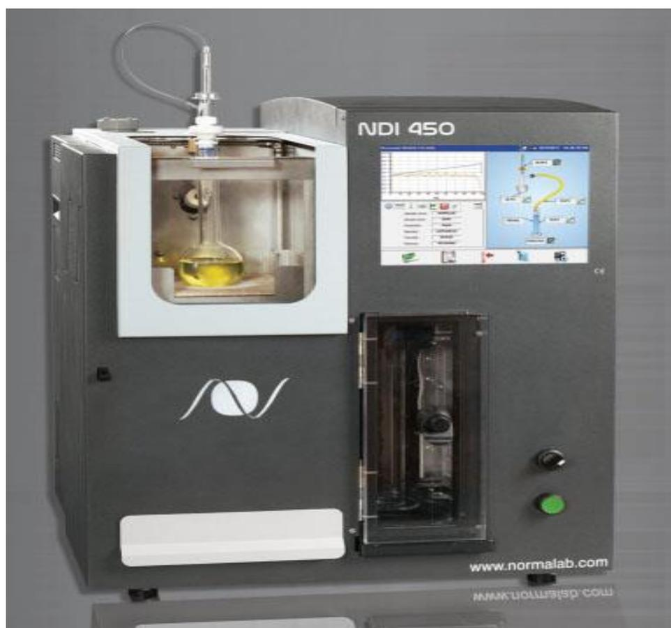
Figure IV.9 : Appareil de Distillation ASTM D86
