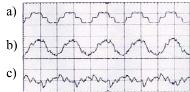
a) nonlinear load current ; b) source current after harmonic current compensation ; c) active filter current ;
