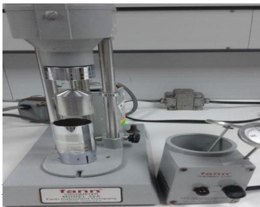
**FigureIV.4:** Rhéomètre FANN
